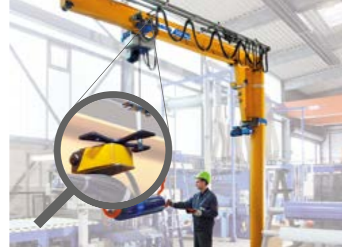
Limit switch for cross travel (Fig. 8)
