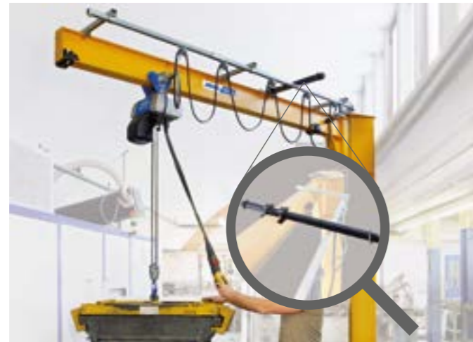
Slewing limit stop - bumper rod (Fig. 4)
