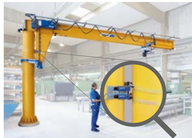
Slewing limit switch, VS (Fig. 6)
