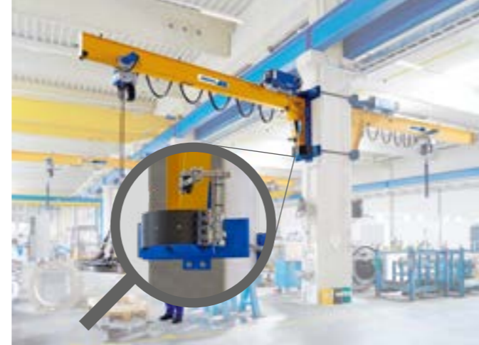
Slewing limit switch, VW (Fig. 7)
