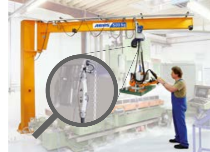
Jib crane with additional power socket and plug on hoist (Fig. 13)
